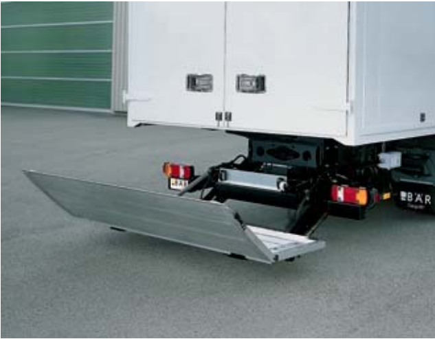
Manual unfolding of the platform spring assisted.
