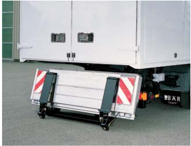
Mechanical setting up of the platform package by lowering it.
